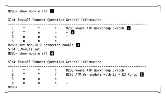
Figure 37. Sample Screen to Check the Physical Installation
